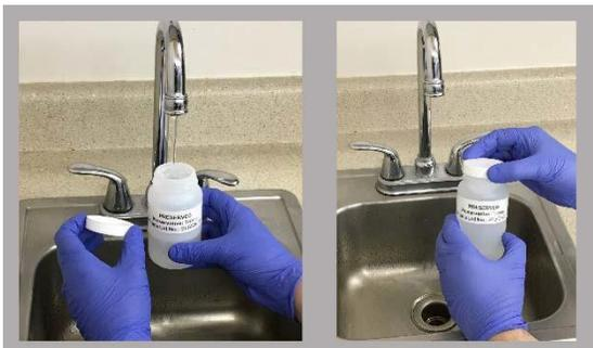
7. Fill the sample bottle to the fill line. If there is no fill line, fill the bottle up to the bottom of the neck. **Be careful to not let the water overflow.** Close the bottle.
