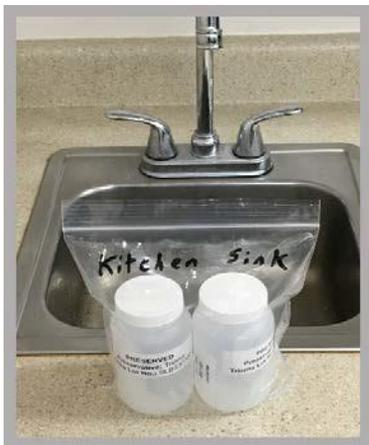
11. Put on a new pair of disposable gloves. In the cooler should be a full bottle labeled “PFAS-free water” or “D.I. water.” Leave the bottle in the cooler, but remove and discard the bottle lid. Open the lid of the bottle labeled “field blank.” Have your partner hold the lid with gloves on or set it upside down somewhere clean.
