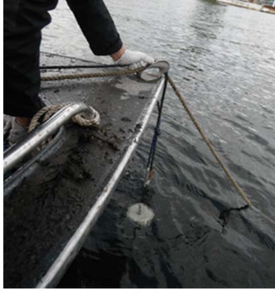
Photograph 1. VOC sampler collecting water sample at 0.15 m depth.
