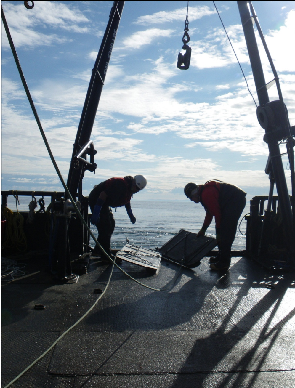
Figure 14 – Deploying Otter Trawl Doors off the Stern of the Norseman II
