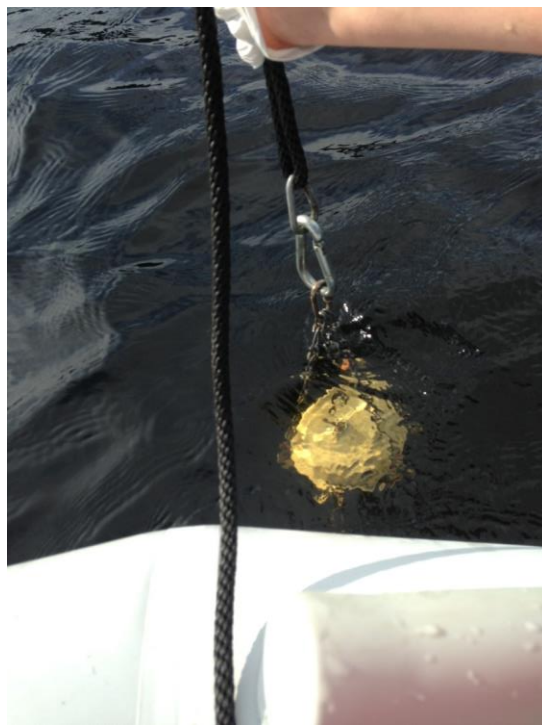
Figure 3: Wildco VOC sampler being lowered into Auke Lake to collect a TAH sample.
