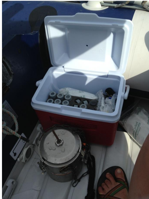
Figure 4: Wildco VOC sampler and VOC sample vials on ice immediately after sample collection.
