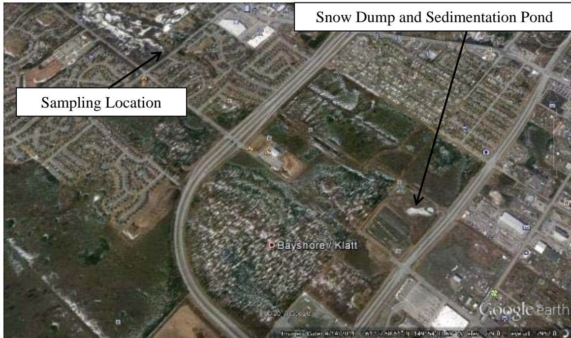
Photograph 1. Aerial view of Campbell Lake Tributary showing the location of the snow dump and sediment basin on the West side of C street and the sampling location on the West side of Victor Road. The tributary flows underground from the sediment basin to Victor Road.
