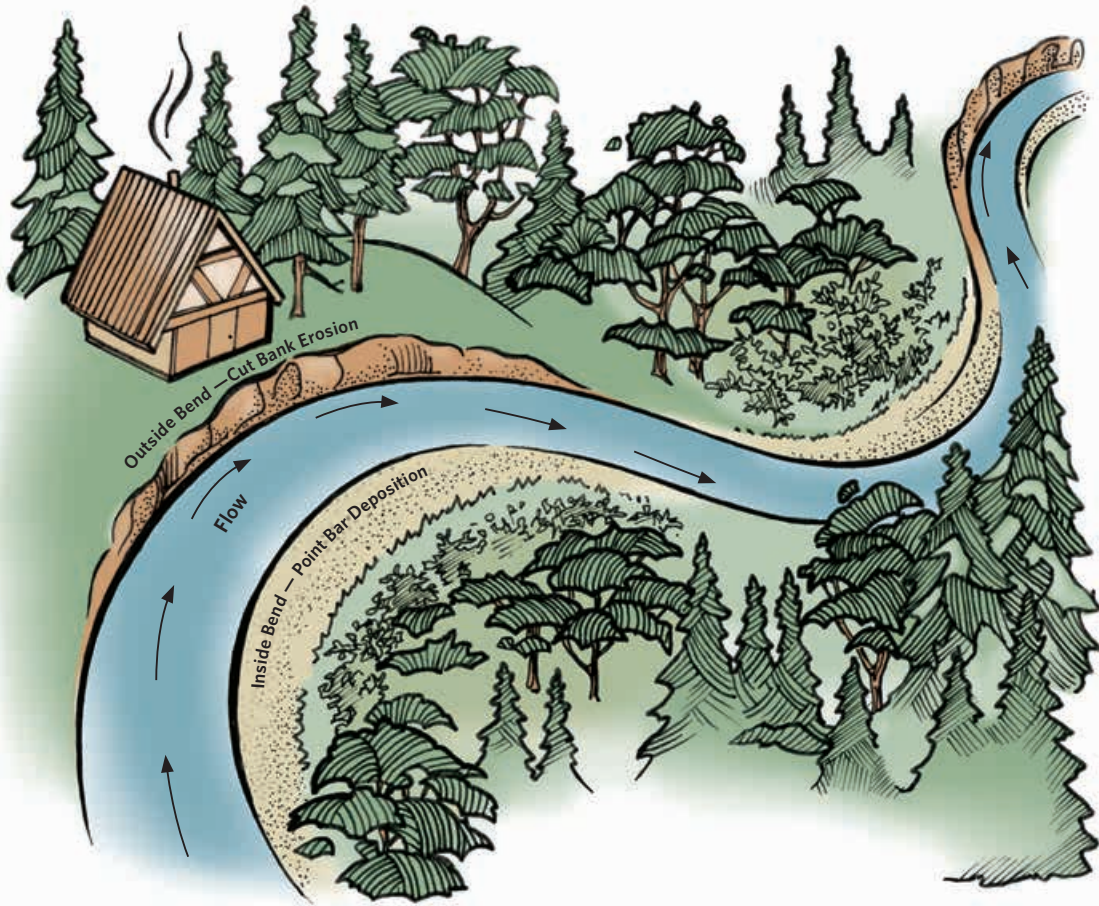
Placement of homes and other structures too close to a river can result in the undermining of the structure over time. Clearing of vegetation also hastens the loss of stream bank from erosion.
