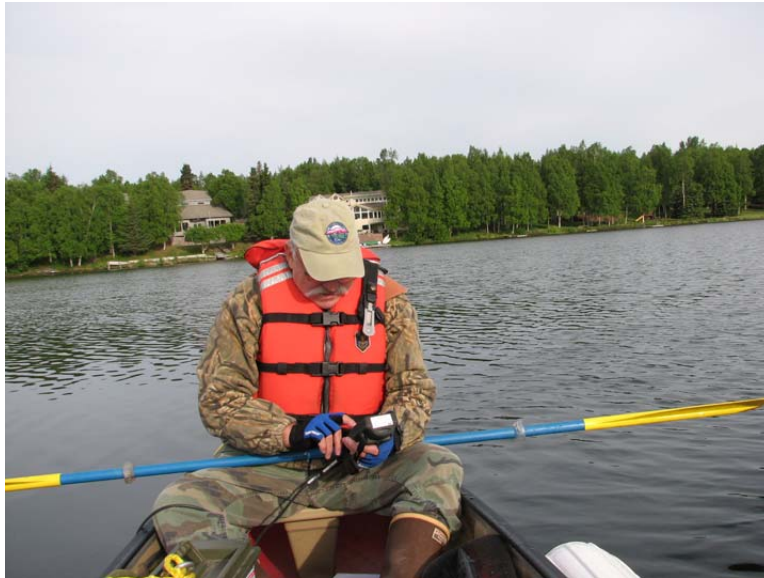
Figure 13. Dr. Thom Eley recording water temperature, pH, and dissolved oxygen with a YSI Professional Plus Instrument on Jewel Lake, June 2010 (Photo by Cherie Northon).
