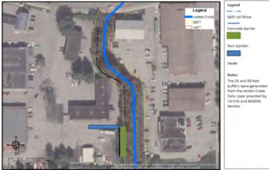
Figure 4. Plan Set showing the fence, rain garden and swale in relation to the Jordan Creek habitat setbacks.
