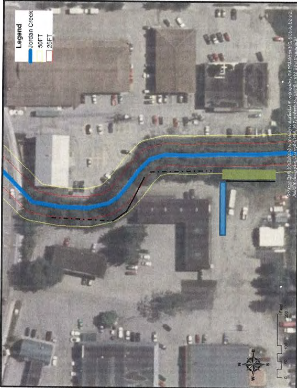
Figure 4. Plan Set showing the fence, rain garden and swale in relation to the Jordan Creek habitat setbacks.
