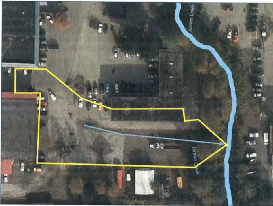
Figure 1. The Edward K Thomas Building showing the area contributing to the stormwater discharging to Jordan Creek in yellow and the current flowpath of stormwater discharging into the creek.
