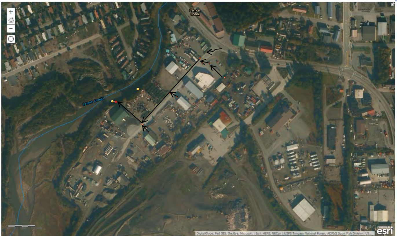
Figure 2. Map of the Concrete Way sub-drainage, showing the mapped stormwater structures (orange dots) and the outfalls identified during CBJ's 2008 inventory (yellow dots). The subdrainage discharge point to Lemon Creek is shown in red.
