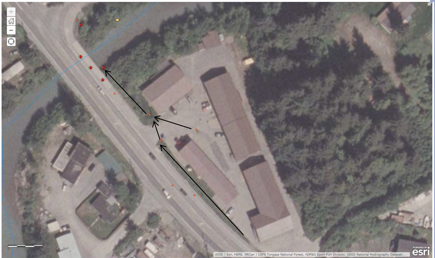
Figure 3. Map of the Space Unlimited and Lemon Creek Bridge sub-drainages, showing the mapped stormwater structures (orange dots). Outfalls to Lemon Creek are shown in red. Flow through the Space Unlimited subdrainage is shown by the arrows. The entire Lemon Creek Bridge subdrainage consists of overland flow to the outfalls on the bridge.
