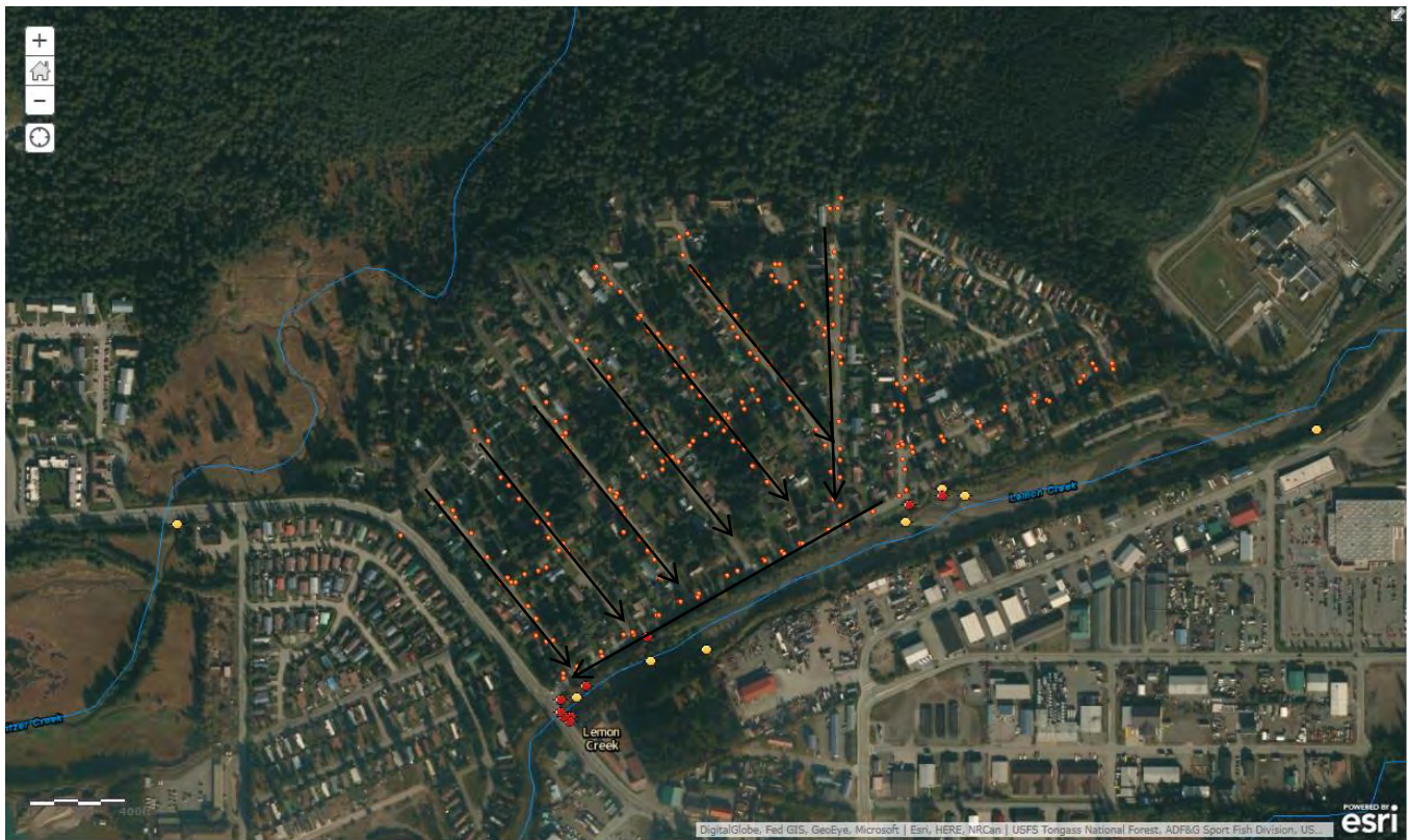
Figure 4. Map of the Pinewood Park Residential sub-drainage, showing the mapped stormwater structures (orange dots). Outfalls to Lemon Creek are shown in red. The outfalls identified during CBJ's 2008 inventory (yellow dots). The general flow through this sub-drainage is shown by the arrows.
