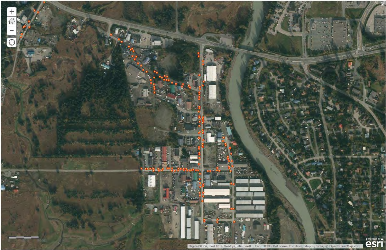
Figure 17. Map of the Industrial Boulevard area. Stormwater mapping revealed that this area does not drain to the Pederson Hill Creek watershed; it appears that this area either slowly drains or flows toward the Mendenhall River. The mapped stormwater structures appear as orange dots.
