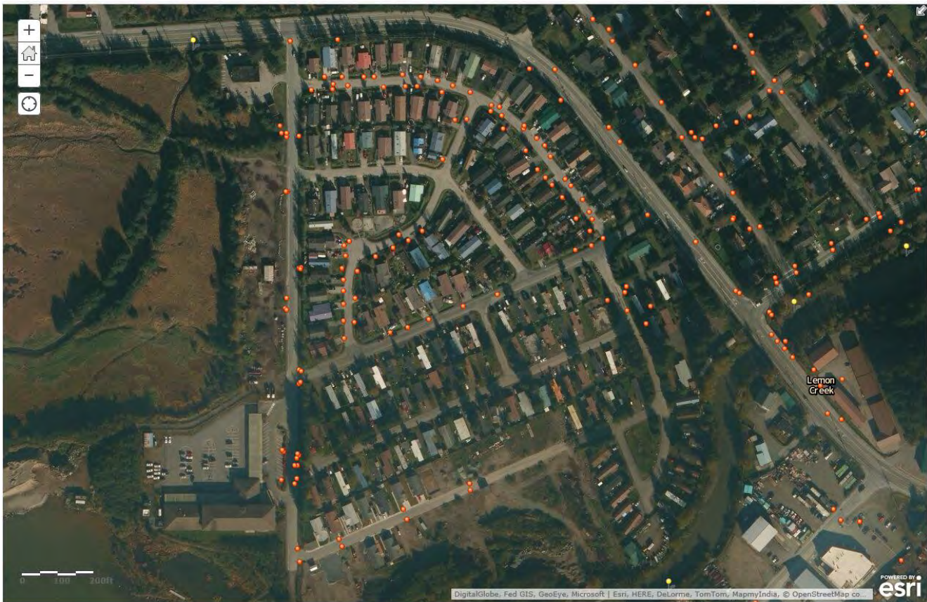
Figure 18. Map of residential area near Switzer and Lemon Creeks. Stormwater mapping revealed that this area does not drain to the Lemon Creek watershed, but to the Switzer Creek watershed. The mapped stormwater structures appear as orange dots.
