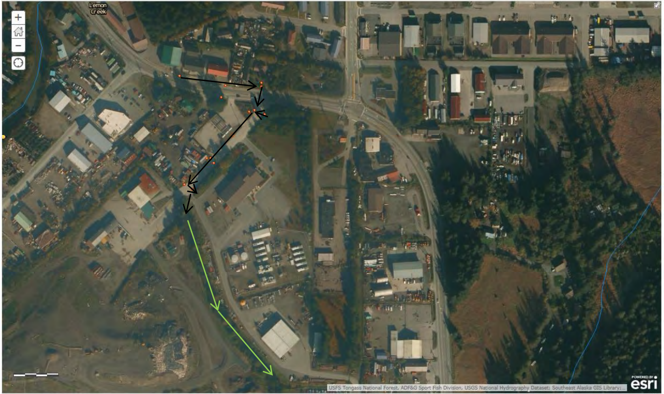
Figure 9. Map of Glacier Highway – Tongsgard Court sub-drainage, showing the mapped stormwater structures (orange dots). The observed flow through the storm sewer system in this subdrainage is indicated by the black arrows. The green arrow shows the hypothesized flow through the swale that borders the landfill, which is based on the landfill’s plan sets.
