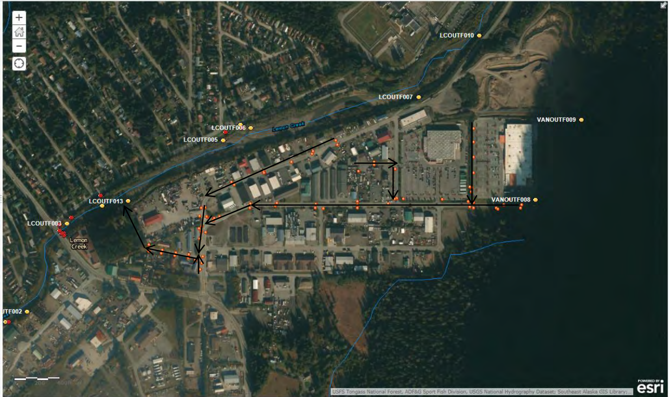
Figure 6. Map of the Aisek sub-drainage, showing the mapped stormwater structures (orange dots). The outfall LCOUTF013 identified during CBJ's 2008 inventory (yellow dot) is the discharge point for this subdrainage. The general flow through the storm sewer system is indicated by the arrows.
