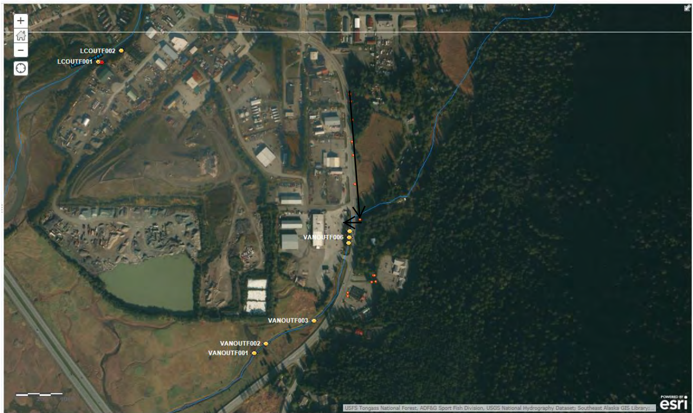
Figure 11. Map of the East Ditch sub-drainages, showing the mapped stormwater structures (orange dots) and the outfalls identified during CBJ's 2008 inventory (yellow dots). The general flow through the subdrainage is shown by the arrows.
