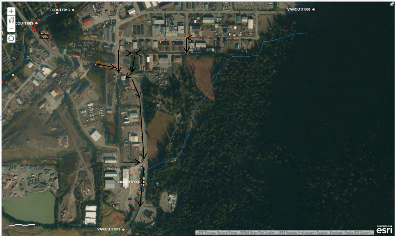
Figure 10. Map of the West Ditch and East Ditch sub-drainages, showing the mapped stormwater structures (orange dots) and the outfalls identified during CBJ's 2008 inventory (yellow dots). The general flow through the subdrainage is shown by the arrows.
