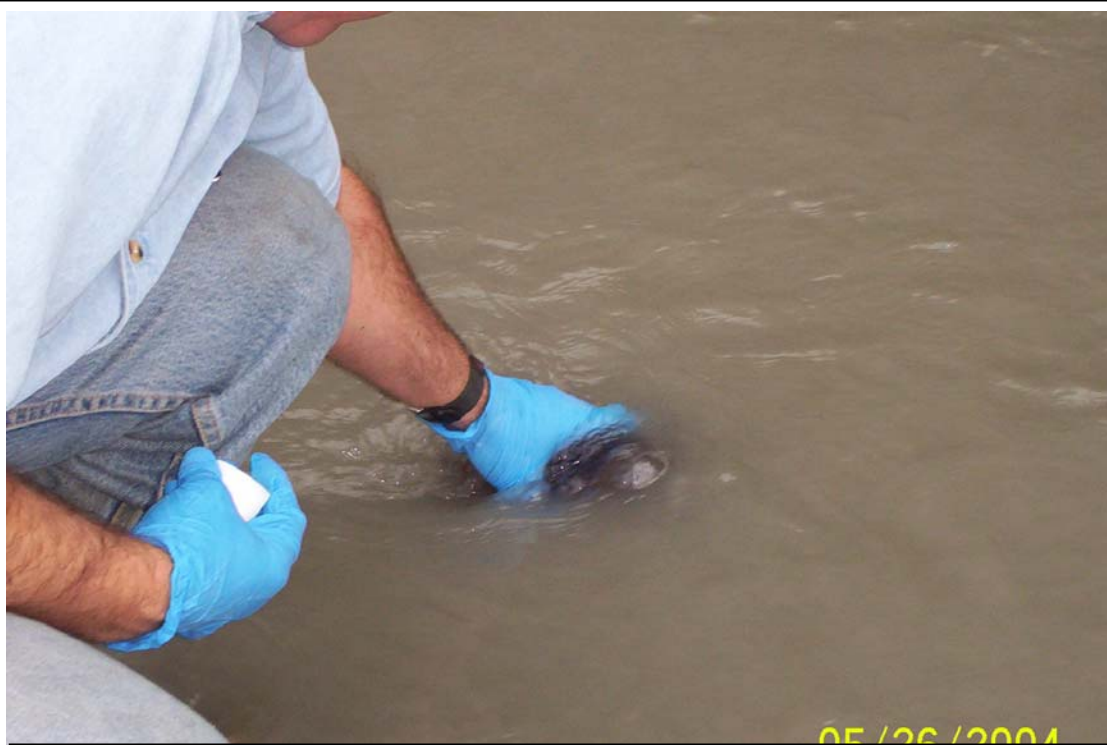
Photo #20 – Close up view of filling a surface water sample container. (5/26/2004)
