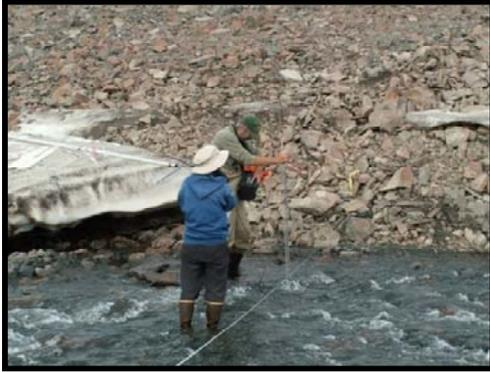
Figure 9. Measuring stream discharge.
