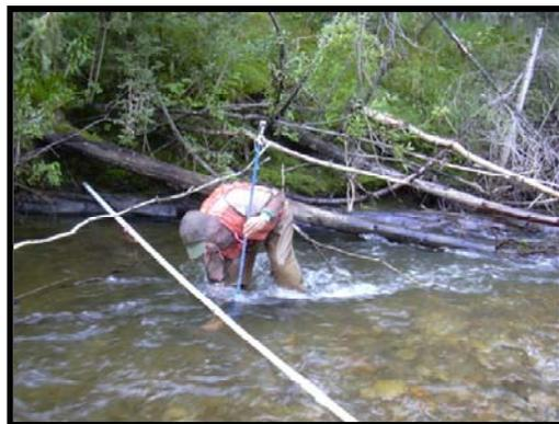
Figure 8. Measuring depth and substrates along a channel transect.
