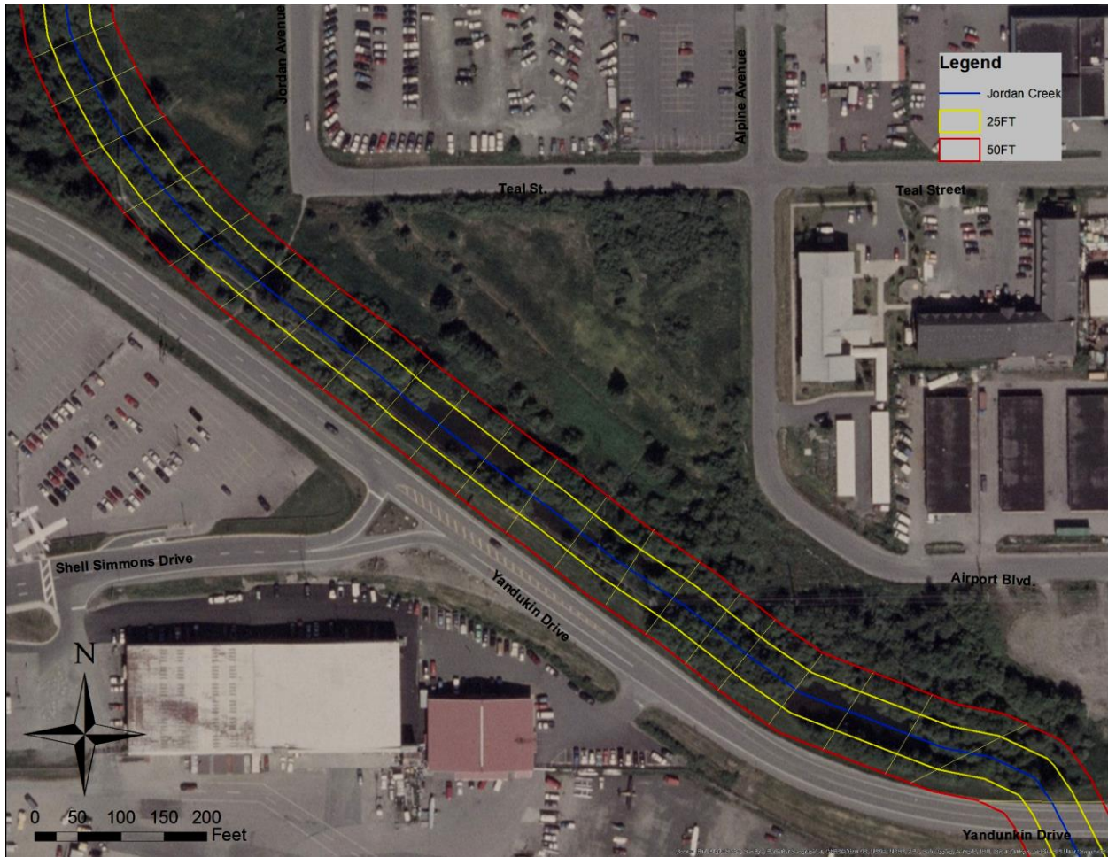
Figure 11. The 25 and 50-foot streamside setbacks along Reach 5 of lower Jordan Creek (yellow and red, respectively). The stream flows northwest to southeast, with the right bank adjacent to Yandukin Drive. This is for visualization purposes only; breaks between stream sections were estimated using GPS waypoints and setbacks projected using the buffer tool in ArcGIS.
