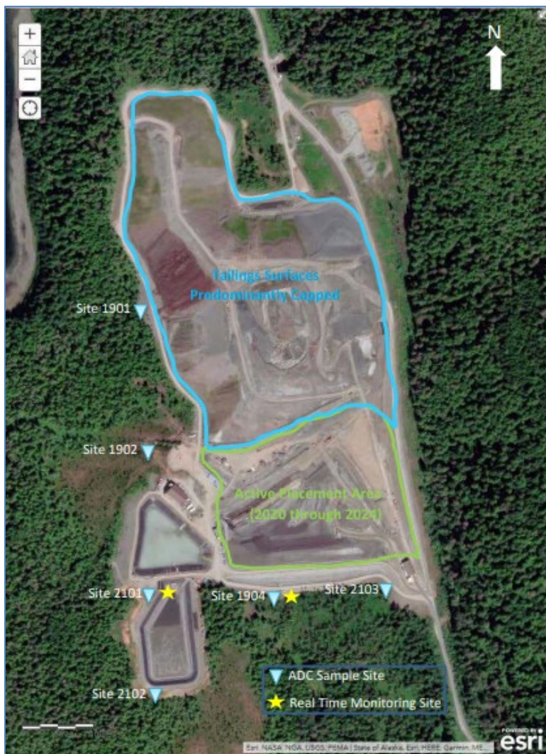
Figure 5. Dust monitoring, including Atmospheric Depositional Container (ADC) and real time monitoring locations
