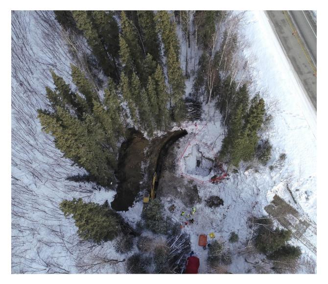
Aerial view of spill site on March 16 2018, facing down. The area known contain affected soils and groundwater is located inside the red exclusion tape. Interception tactics had been completed at this time, and clean soils stockpiled adjacent to the trench (Photo/ADNR).
