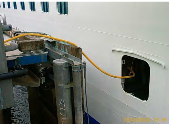
Photo 4: GW offload hose in Juneau 1
