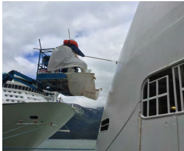
Photo 10: Painting, with drop cloth protection
