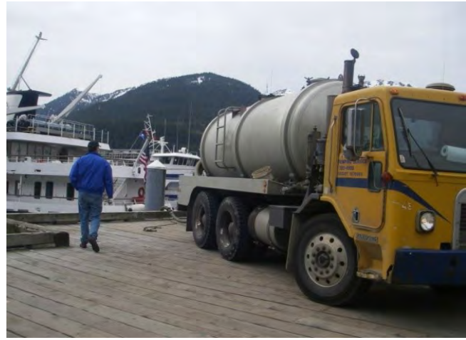
Photo 3: Sewage Offload by tank vacuume truck
