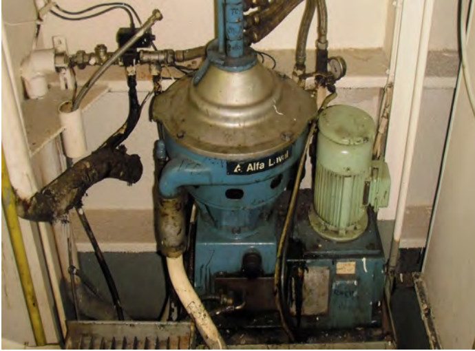
Photo 56: OWS separator (dynamic)
