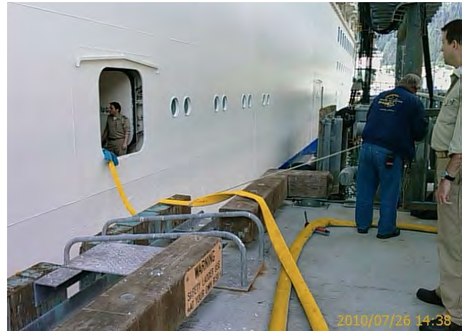
Photo 5: GW off load hose in Juneau 2
