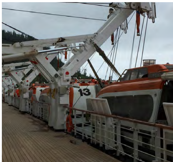
Photo 63: Lifeboats, extended for drill
