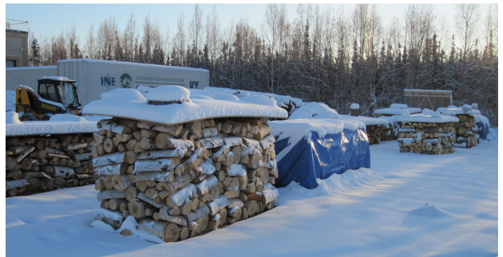
Although none of the fall harvest fully cured over one winter, split birch firewood stored in a simulated wood shed (shown here) dried the most, to a 30% moisture content.
