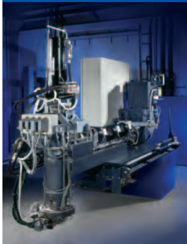
Fig. 9.1 · Suction blow molding machine (photos from SIG – Kautex)
