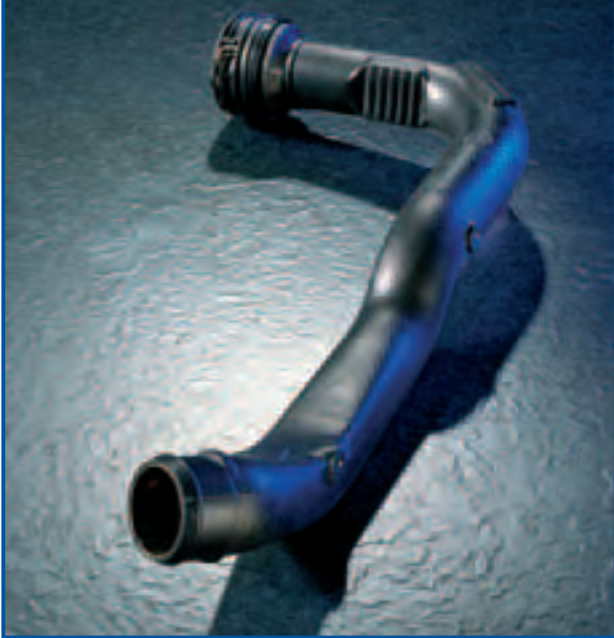
Fig. 9.2 · Blow molded air duct for turbo-charged diesel engines with hot plate welded connecting flange (Mann & Hummel)
