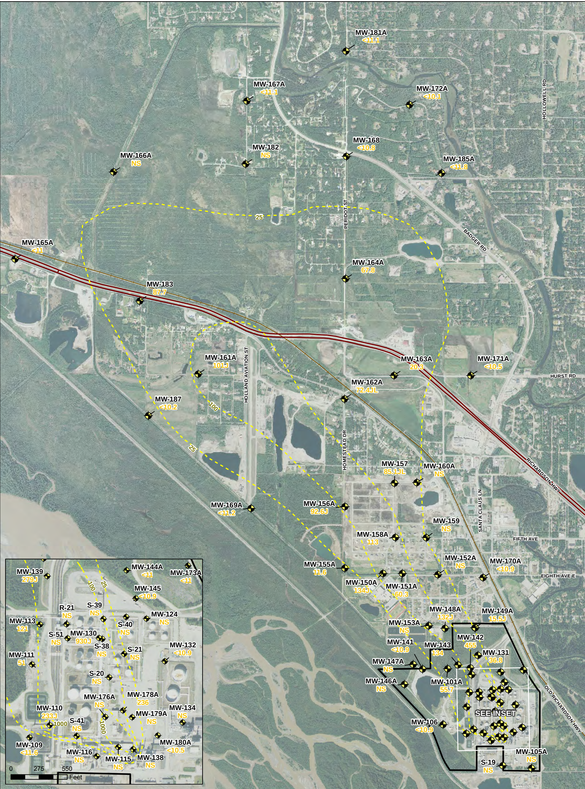
Figure 92 SULFOLANE CONCENTRATIONS IN GROUNDWATER AT THE WATER TABLE FIRST QUARTER 2011 North Pole Refinery Flint Hills Resources Alaska, LLC
