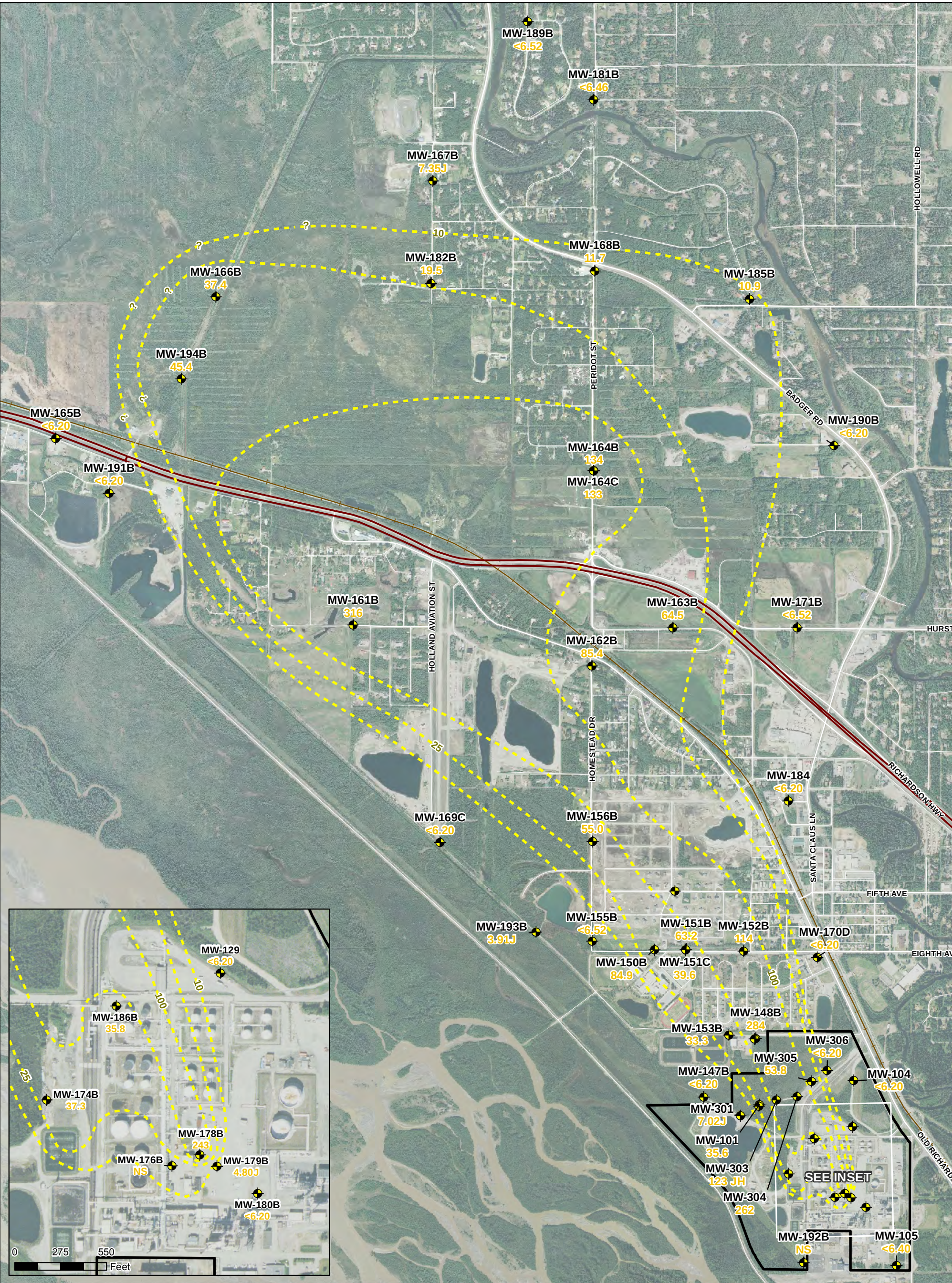
Figure 104 SULFOLANE CONCENTRATIONS IN GROUNDWATER 10-55' BELOW THE WATER TABLE FOURTH QUARTER 2011 North Pole Refinery Flint Hills Resources Alaska, LLC
