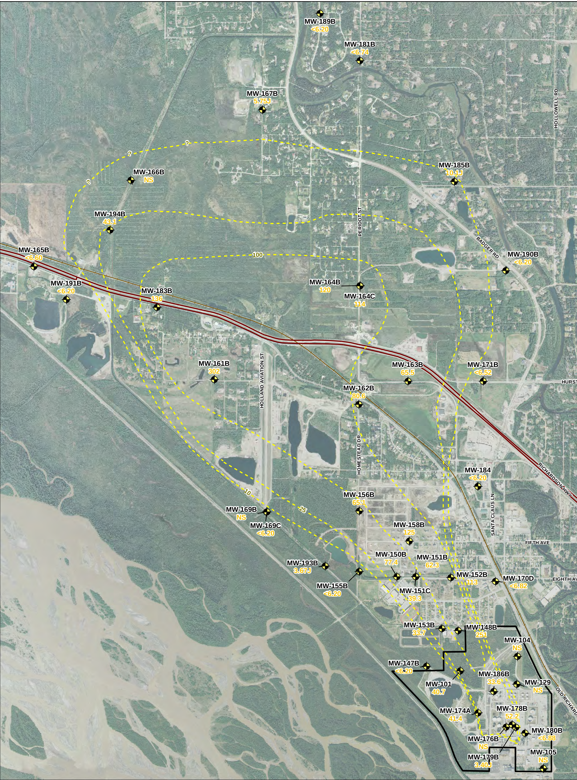
Figure 100 SULFOLANE CONCENTRATIONS IN GROUNDWATER 10-55' BELOW THE WATER TABLE THIRD QUARTER 2011 North Pole Refinery Flint Hills Resources Alaska, LLC
