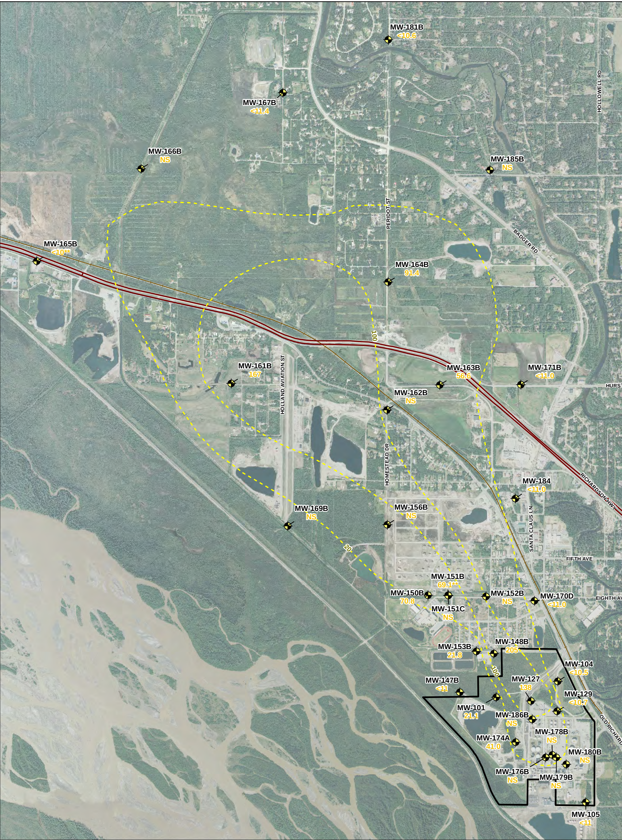
Figure 97 SULFOLANE CONCENTRATIONS IN GROUNDWATER 10-55' BELOW THE WATER TABLE SECOND QUARTER 2011 North Pole Refinery Flint Hills Resources Alaska, LLC
