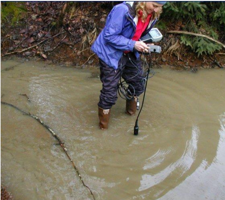
Figure 9b. Photo of sampling in situ water quality parameters in Duck Creek at site DC-B on 4/7/05 when active construction of the Nancy Street wetlands was underway immediately upstream of the site. Notice the extremely turbid coloration of the water.
