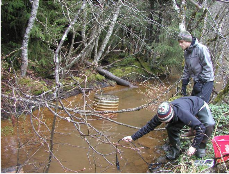
Figure 10. Sampling at site DC-A in April, 2006. The thick coating of iron floc on the streambed is easily disturbed by any activity (including sampling) in the stream. Caution is taken to avoid introducing re-suspended floc into the turbidity and TSS sample bottles, but this is not always possible.
