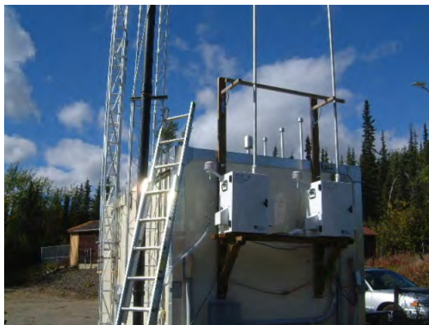
Figure 3. Partisol samplers installed at IMPROVE monitoring site at Denali NPP. IMPROVE inlets are visible on the far side of the shelter.
