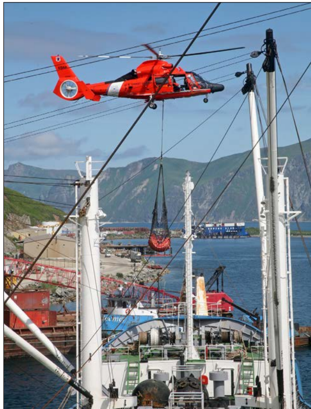
Photograph mh-8. 15-ft. clearance to obstacles and a deck free of debris are required.
