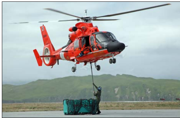
Photograph mh-4. USCG ground crew hooking ETS MK 105 pendant to hovering helicopter.
