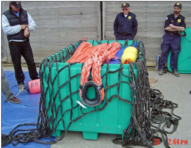
Photograph mh-1. ETS (less than 50,000 DWT system) in cargo net lined prepared for helicopter deployment.
