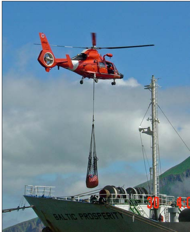
Photograph mh-6. USCG helicopter delivering ETS to the ship's bow; no deck crew on bow of ship.
