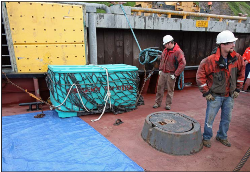
Photograph mt-1. ETS delivered to rescue tug at dock and lashed to deck with "Deploy From Here" corner to the aft and inboard.
