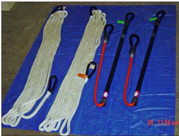
Photograph mh-5. Helicopter pendants and slings stored with large ETS at the DOT Airport Hangar.
