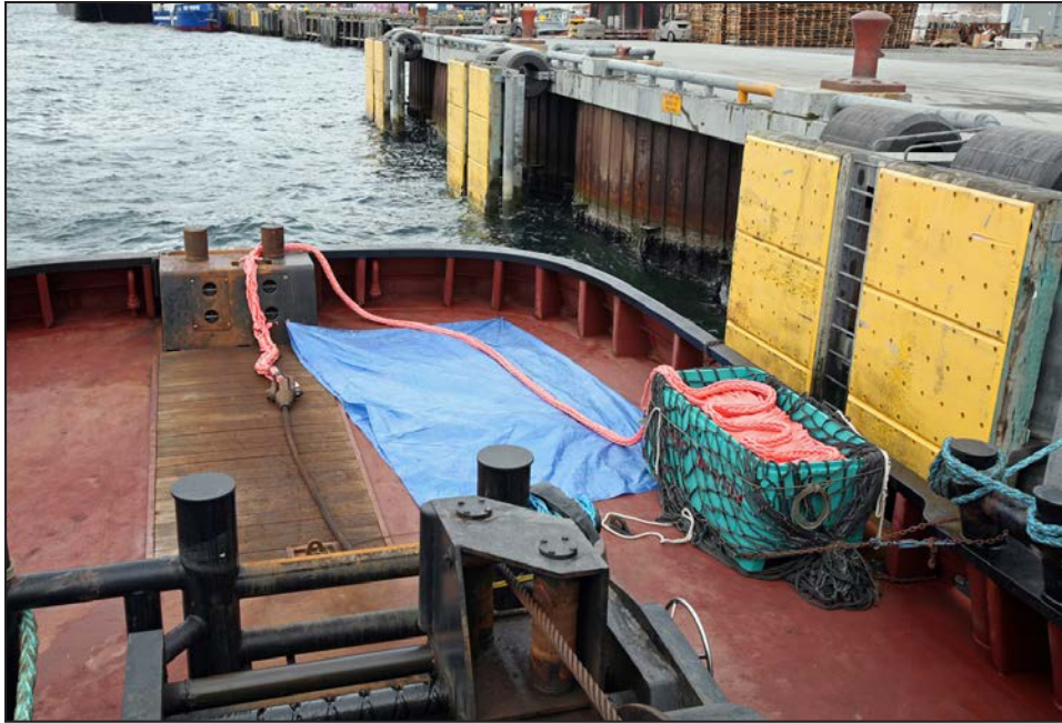
Photograph mt-2. ETS Tow Line shackled to tug's tow wire.
