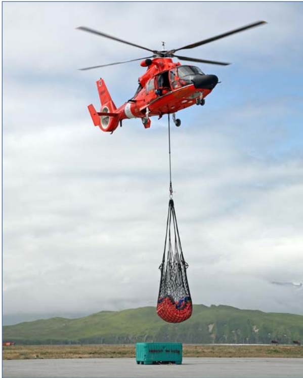
Photograph mh-5. USCG helicopter lifting ETS and cargo net from storage tote/cage.
