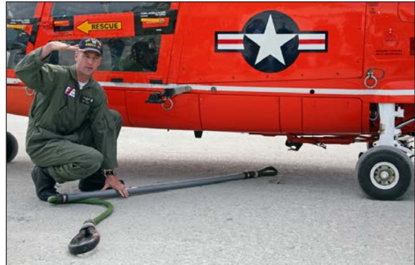
Photograph mh-2. Aircrew member demonstrates attaching the pendant to the cargo release hook.
