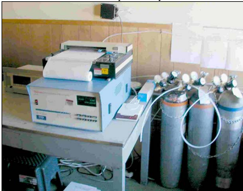
Figure III.B.4-1 TECO 48 CO Analyzer with Strip Chart Recorder and Data Acquisition System
