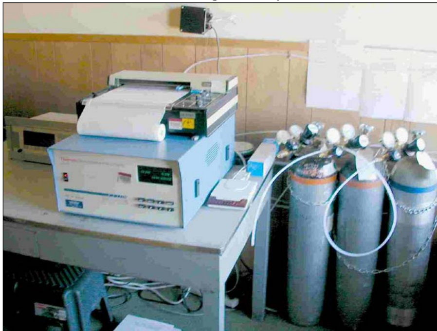
Figure III.B.4-1 TECO 48 CO Analyzer with Strip Chart Recorder and Data Acquisition System
