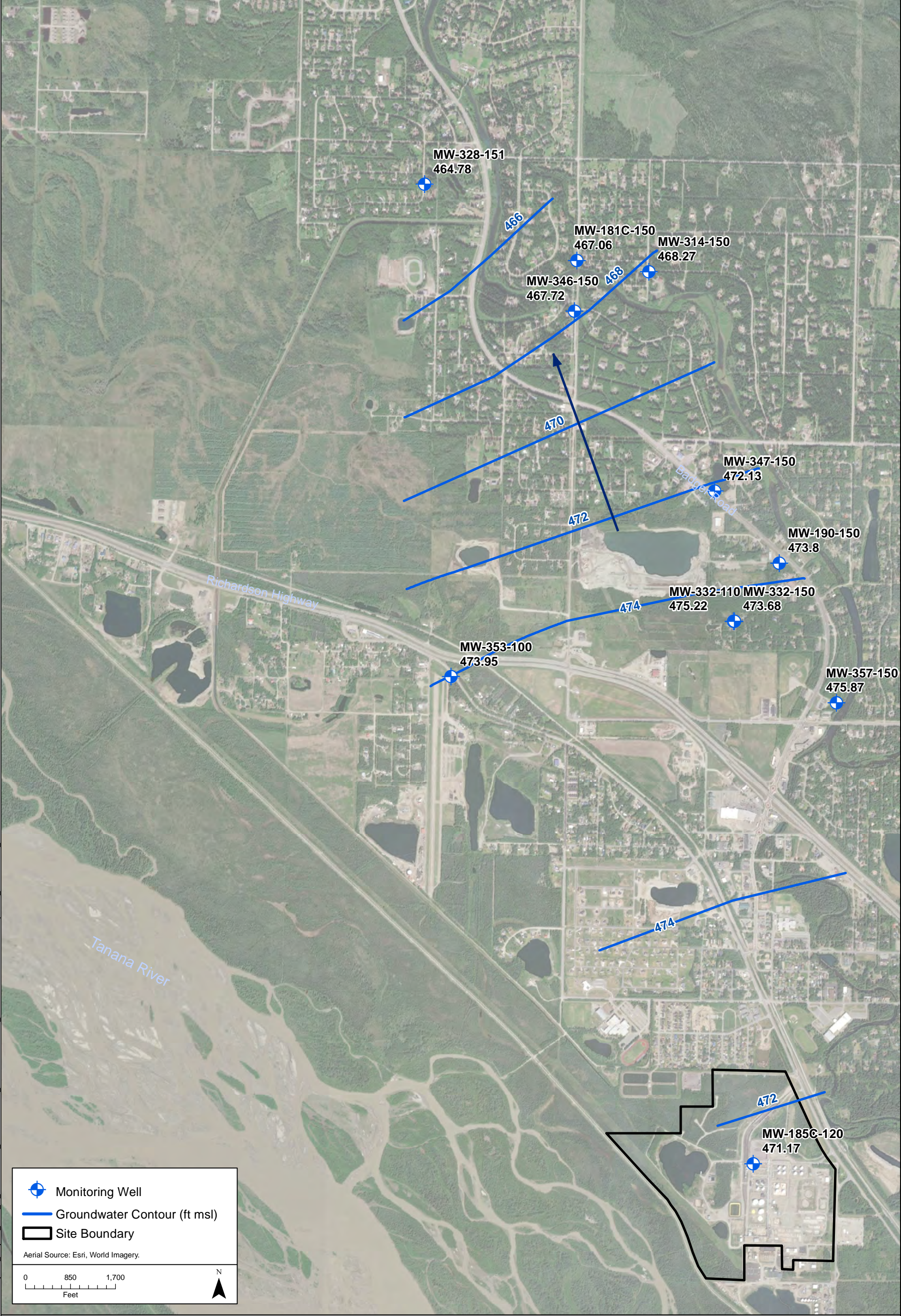
Figure 7. Groundwater Contour Map (Offsite Wells) Zone 3 (90-150 ft) December 2020
