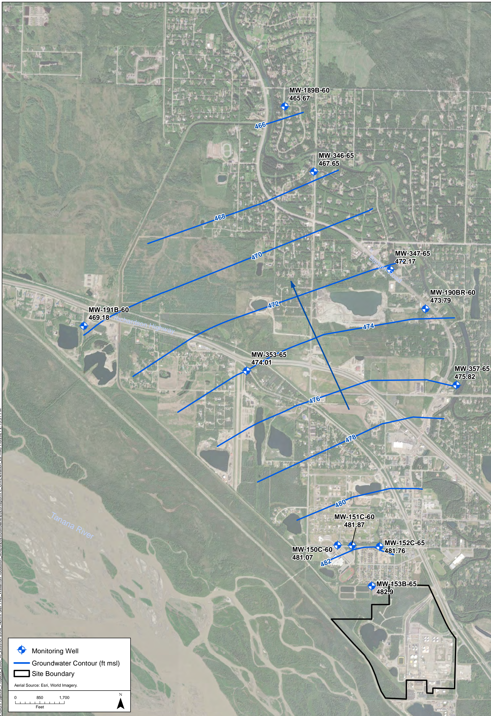
Figure 6. Groundwater Contour Map (Offsite Wells) Zone 2 (55-90 ft) December 2020
