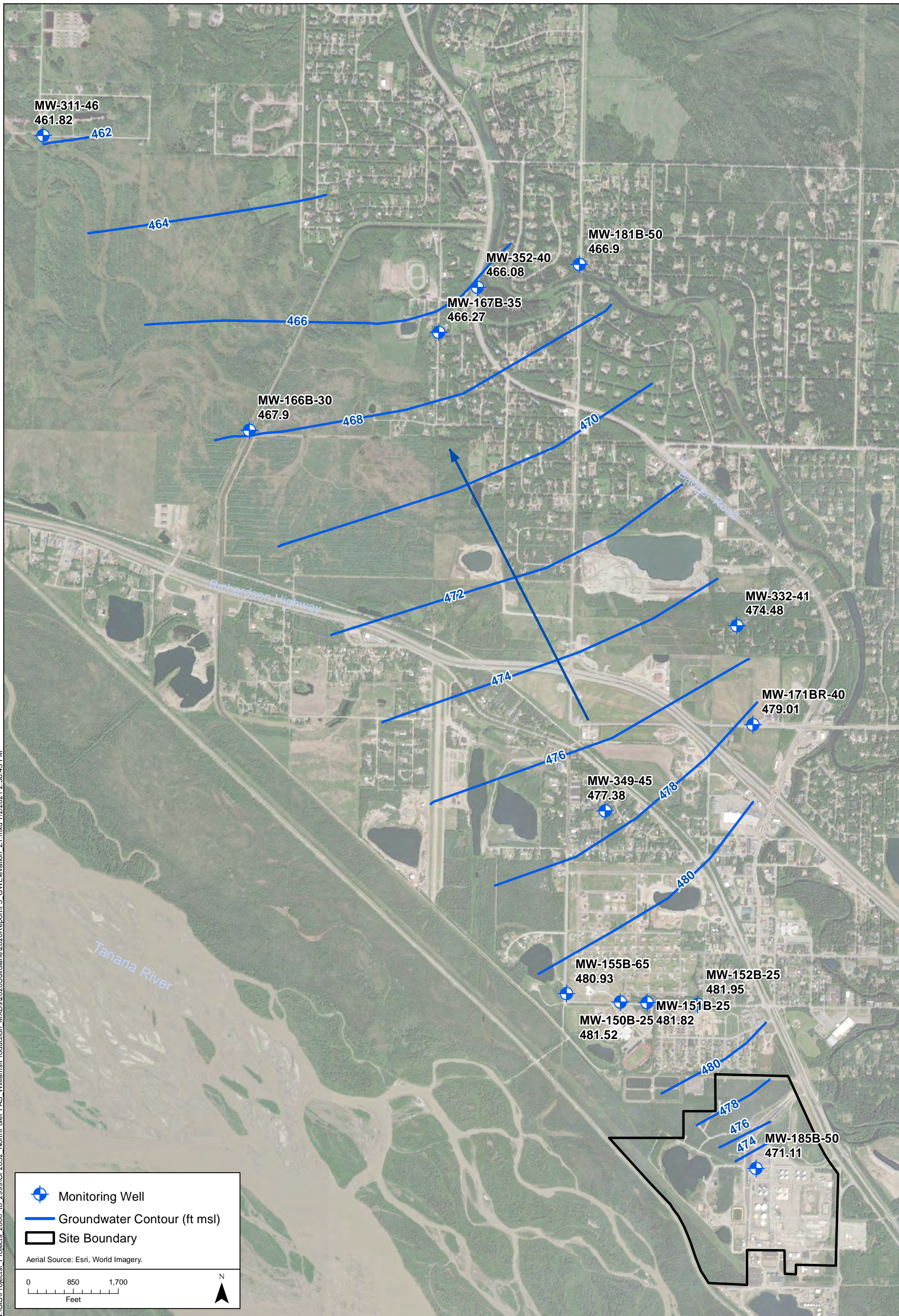
Figure 5. Groundwater Contour Map (Offsite Wells) Zone 1 (10-55 ft)
