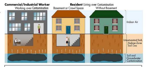
Contamination in the soil and groundwater can take the form of a vapor and travel through soil, entering indoor air through leaks in parts of buildings which are below-ground, like basements and crawl spaces.
