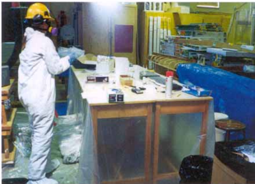
Photo 6: The Aniak Middle School wood shop was used to perform the PCB soil screening tests. The work area surfaces within the wood shop were covered with plastic liners and tarps.
