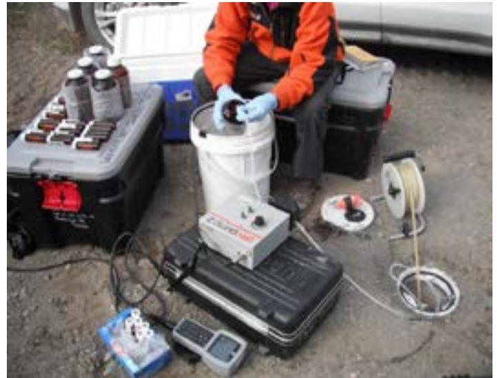
*Taking samples from a monitoring well is part of the site characterization process for this contaminated site in Kotzebou.*
