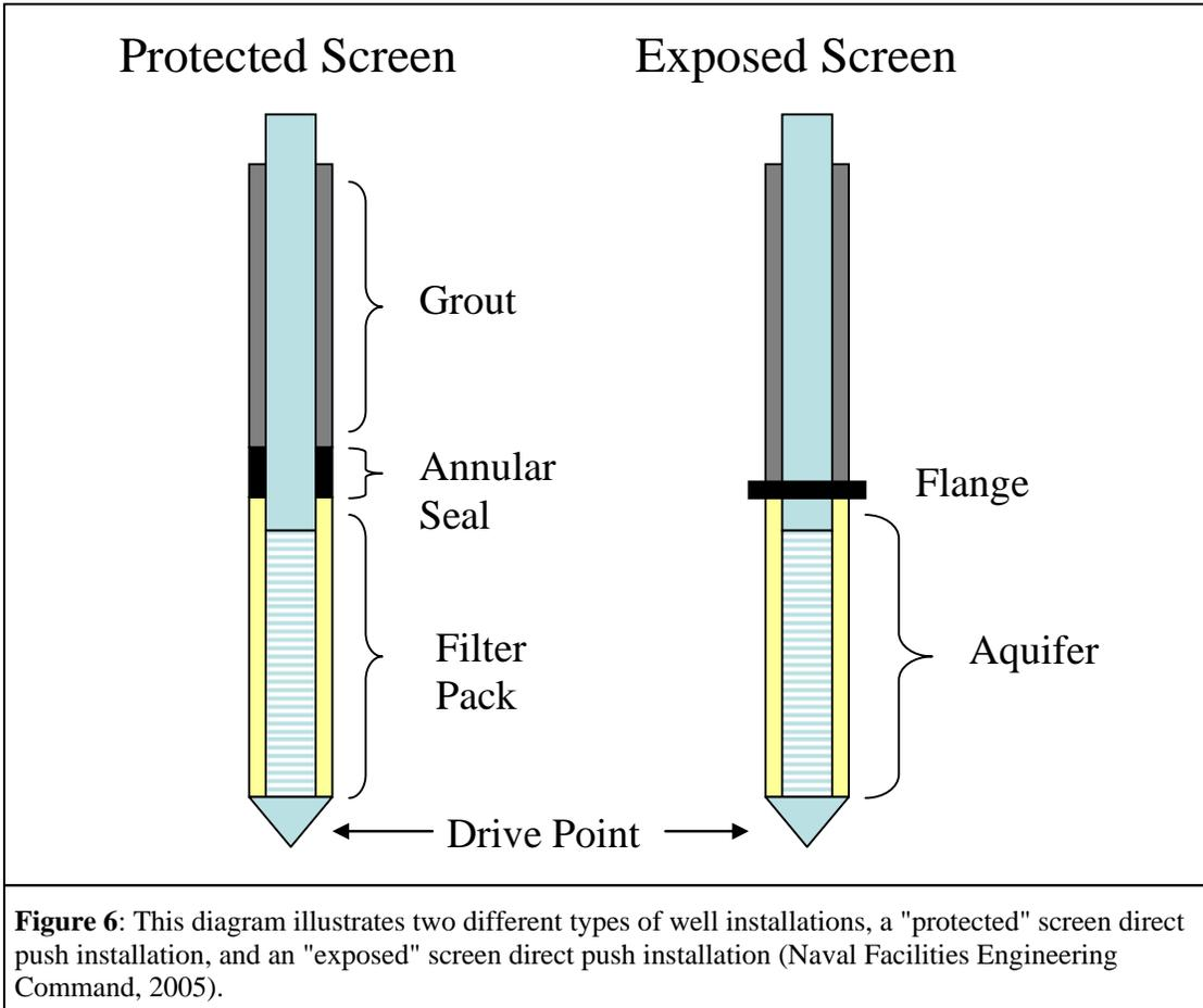
may be approved by DEC for long-term monitoring. The lack of an annular seal in exposed-screen installations may result in the introduction of water or contaminants from the ground surface or across water bearing zones. These type of direct push well are
