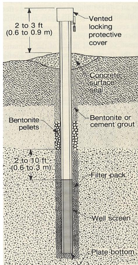
**Figure 1.** Typical Monitoring Well Installation. From Driscoll (1986).
