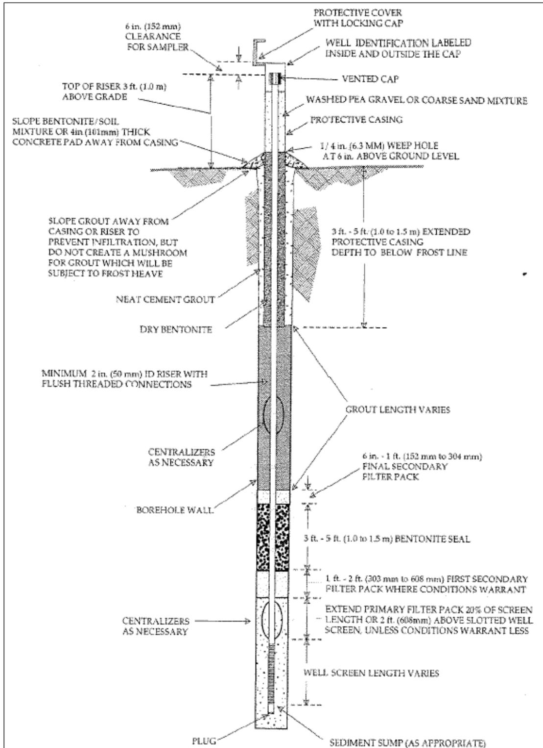
**Figure 5.** Example monitoring well construction design with filter pack. From ASTM 5092 (2005)<sup>2</sup>.
