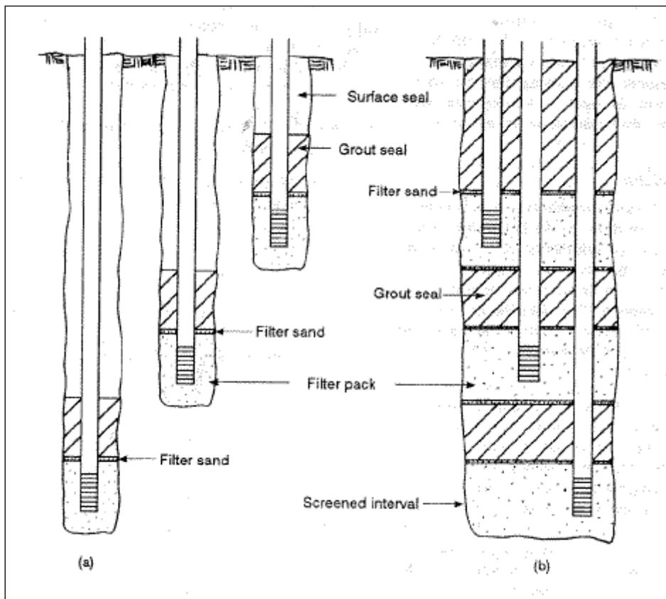
Figure 4. Piezometers installed as (a) clusters, or (b) nested. From EPA (1991).
