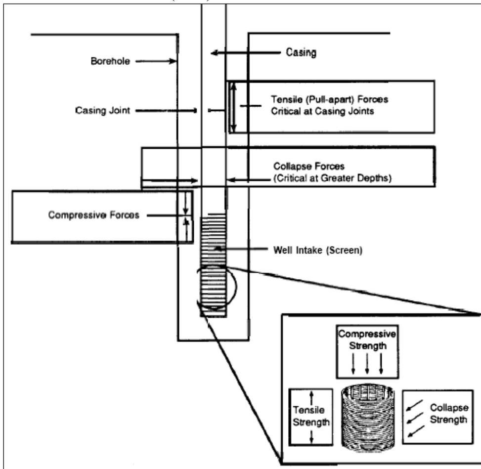
Figure 3. Forces acting on a monitoring well casing during installation. From EPA (1991).
