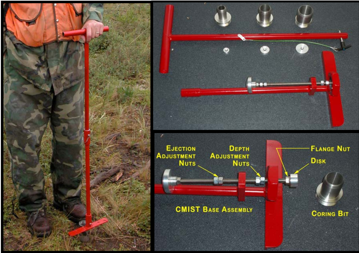
Figure 8-1 - CRREL Coring Device
