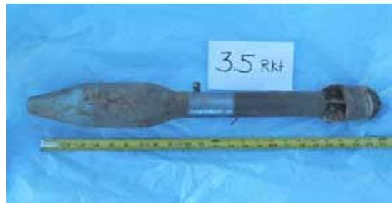
Training rockets like this one do not contain explosives, but the rocket motors had to be inspected for hazardous propellant. (DLA photo, 10/02)
