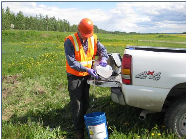
DEC's Dennis Shepard is shown decontaminating a water interface probe during a groundwater monitoring well inspection for an old landfill at the Galena Airport project in the summer of 2012. The landfill is one of several that the Air Force used when the base was active. (DEC photo)
