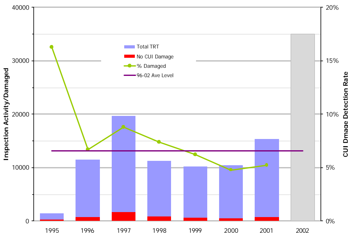
Figure E.2 External Corrosion Activity and Detection Summary
