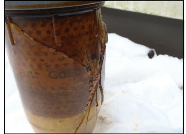
Check your tank for water! Water can corrode a tank from the inside out or cause the fuel filter to crack during cold weather. (Photo)
