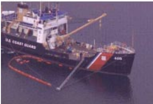
Fig. 3 – The U.S. Coast Guard participated in the on-water booming operations with its Vessel-Operated Skimming System, or VOSS. Courtesy of SONS exercise photography team.
