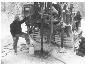
Rig used to drill sentinel wells.
