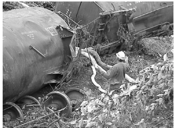
ARRC derailment at Mile 152.8 -- lightering operations
