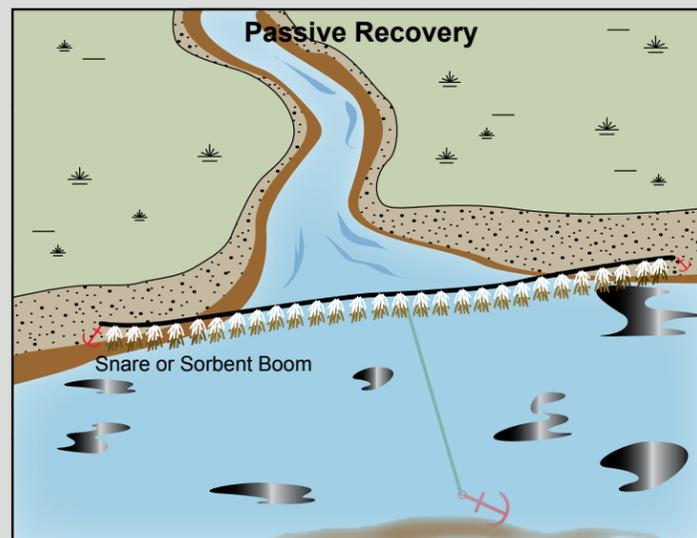
An example of the *Passive Recovery*. Actual deployment should be adjusted for local conditions.
