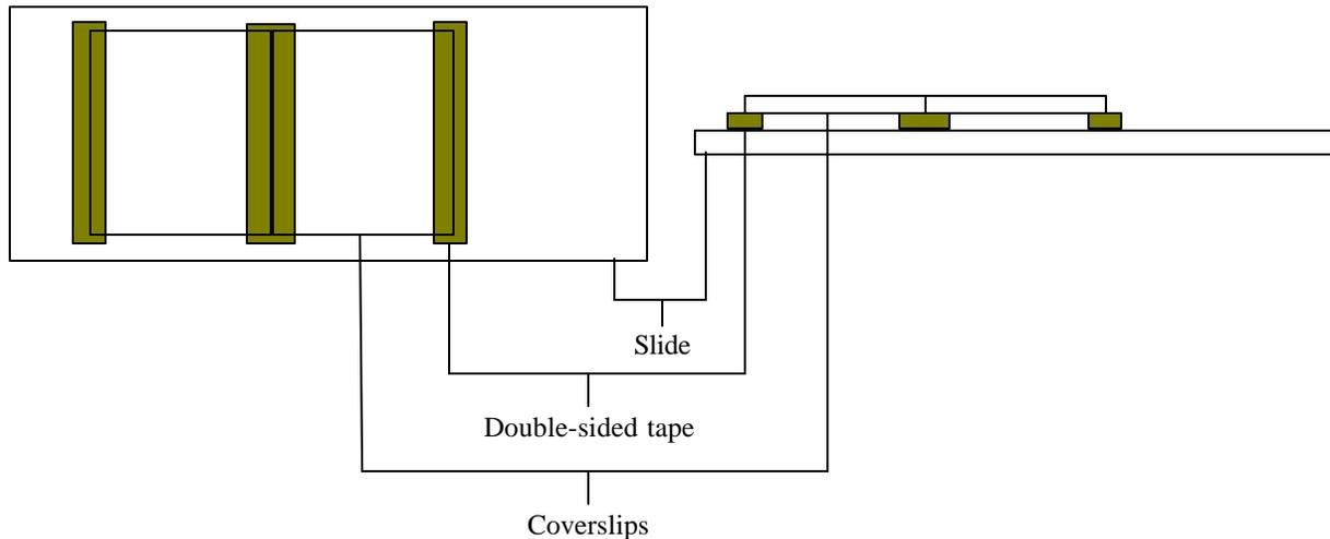
**Figure 2. Schematic Diagram of the Chamber Slide**
