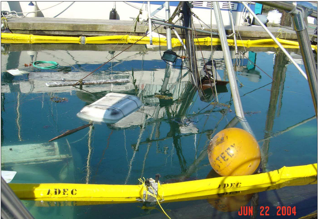
FV Nesteby sunk at its berth in Harris Harbor. Responders have deployed containment boom to capture leaking oil.
