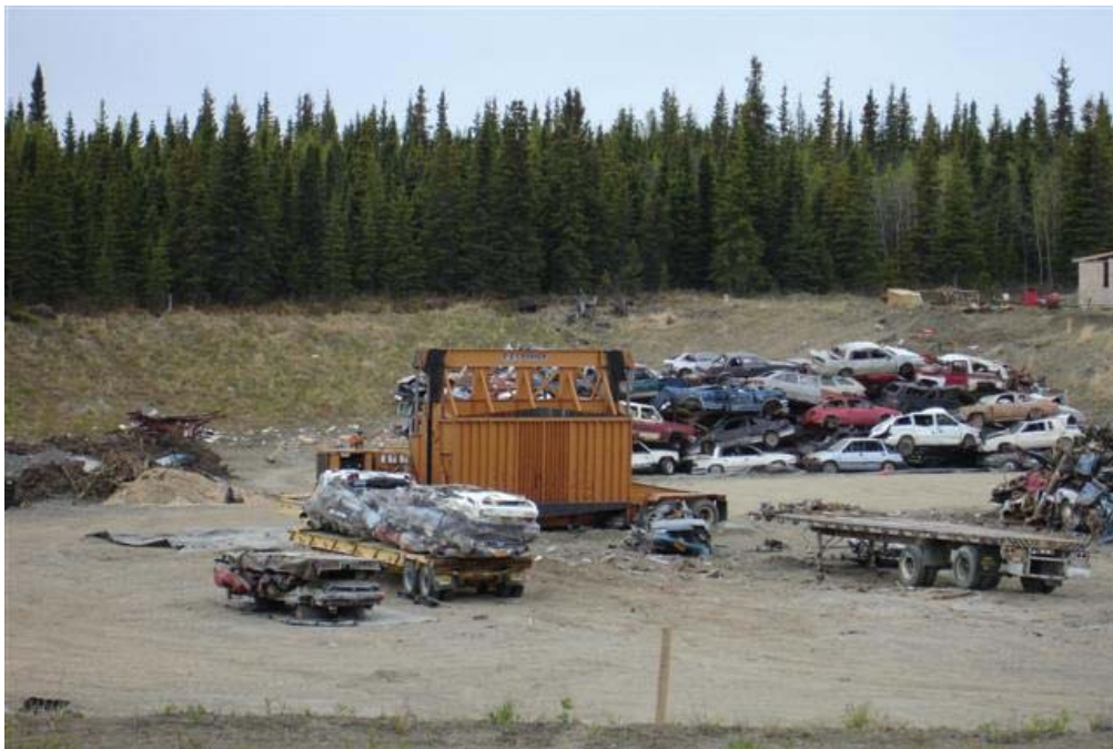
Vehicles are crushed, wrapped and placed on trailers for transport to Anchorage.
