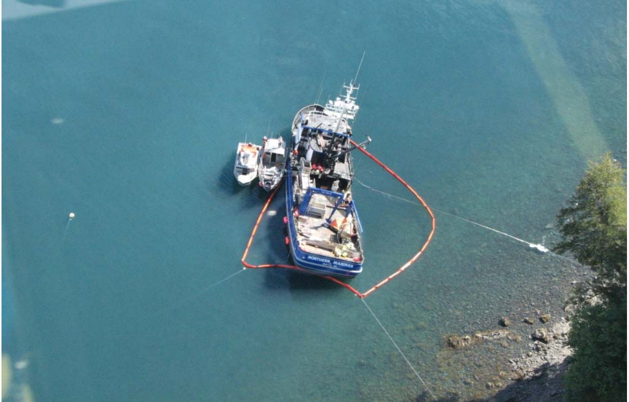
Containment boom was placed around the F/V Northern Mariner to capture any potential spill. Photo provided by the Unified Command.
