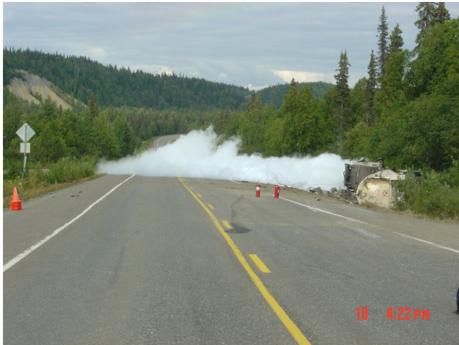
Methane venting from the tanker truck
