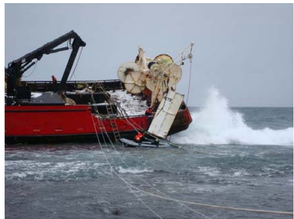
Lashing the transfer hose to support lines.
