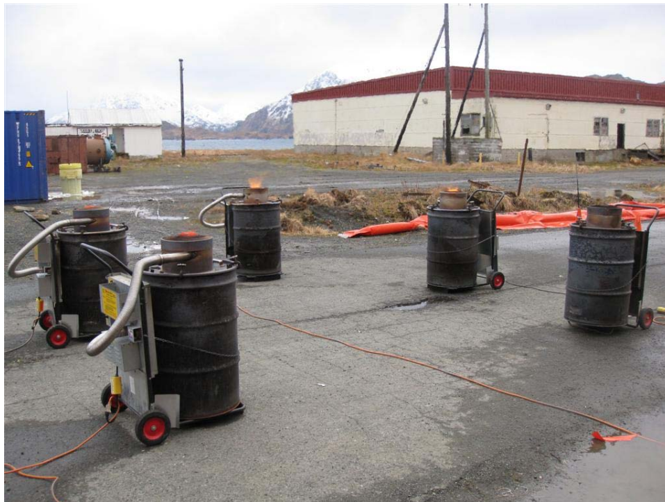
Portable Smart-Ash incinerators burning response-generated solid waste. Photo ADEC/Neil Huddleston
