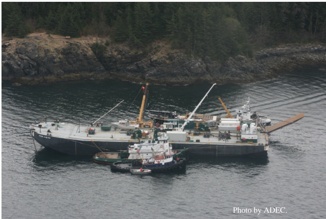
Fuel removal fleet including operations platform, tank barge, and transport vessels off Point Lena.
