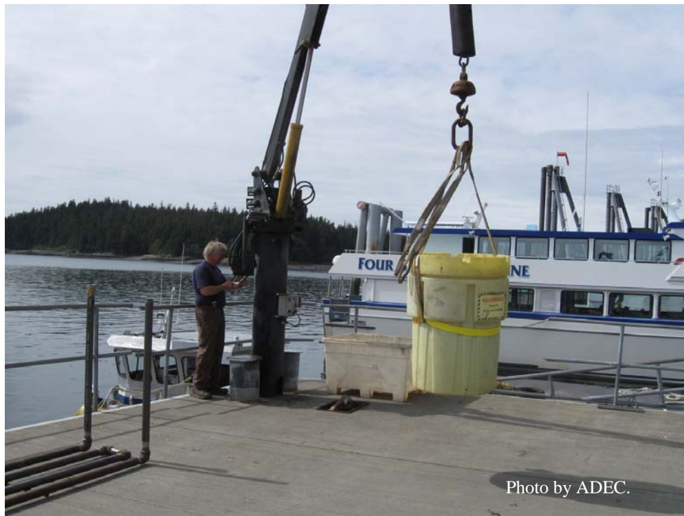
A drum of Petro Sweet within a secondary containment 'over pack' is transferred to a vessel via crane for delivery to the fuel recovery platform. May 4, 2010.
