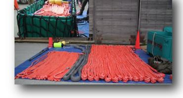
suitable for vessels up to 50,000 DWT and the Alaska Department of Environmental Conservation purchased a system capable of towing vessels greater than 50,000 DWT. A third ETS for vessels greater than 50,000 DWT was purchased in 2009 and is currently staged at the Coast Guard Air Station Kodiak for deployment anywhere in the State.
