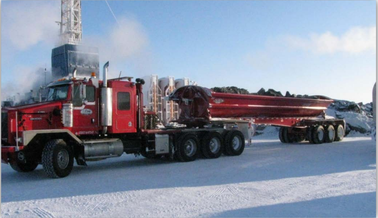
Side dump truck loaded with frozen mud mixed with snow and ice ready for transport to the disposal facility.
