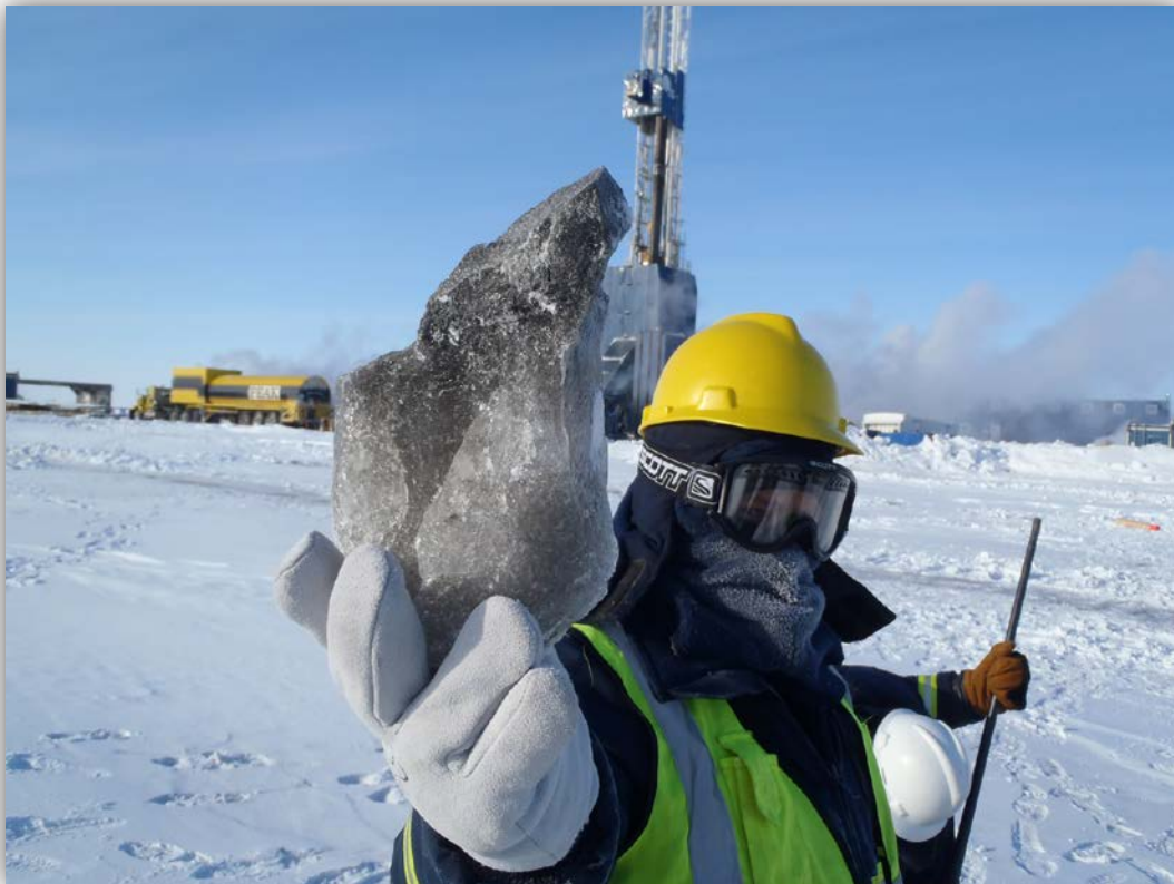
A piece of frozen downhole material ejected out off the pad during the gas kick. ADEC Photo.
