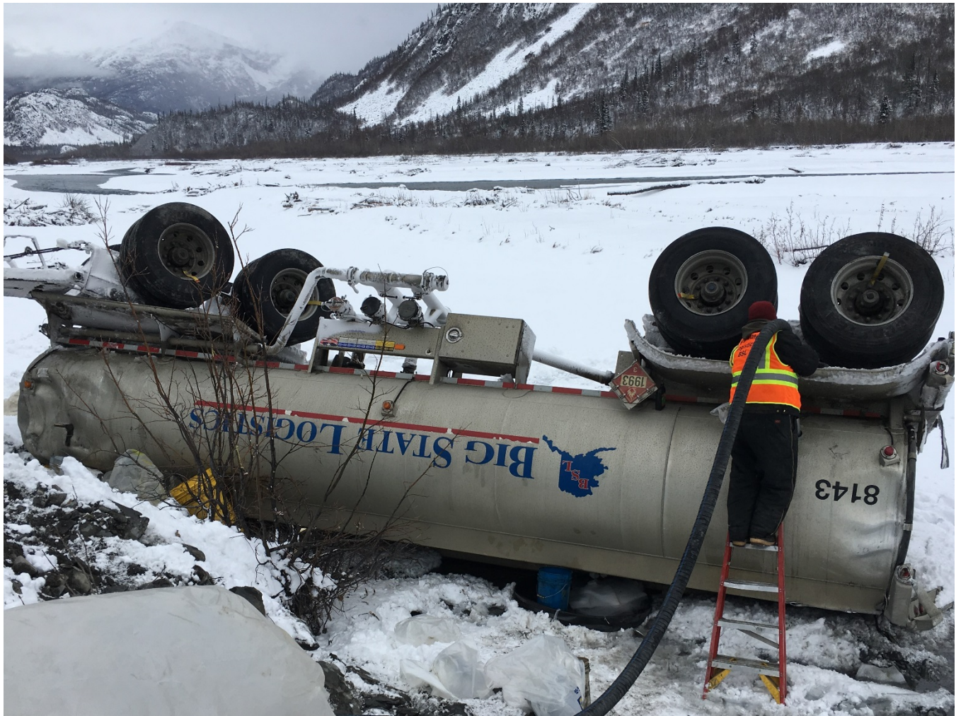
Big State Logistics response crew offloading fuel from a rolled and damaged secondary tank, 42 mile Richardson Hwy. (Photo: Candice Bressler, ADEC)
